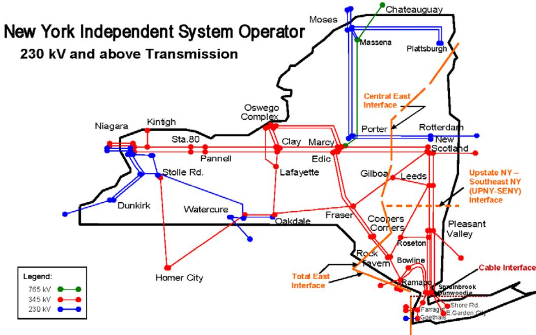
Figure 1: Current New York State Bulk Power Transmission
