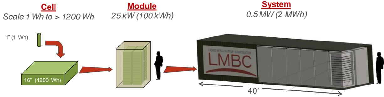
**Conceptual design of LMBC's energy storage solution, representing 0.5 MW / 2 MWh of capacity in the footprint of a 40' shipping container.**
