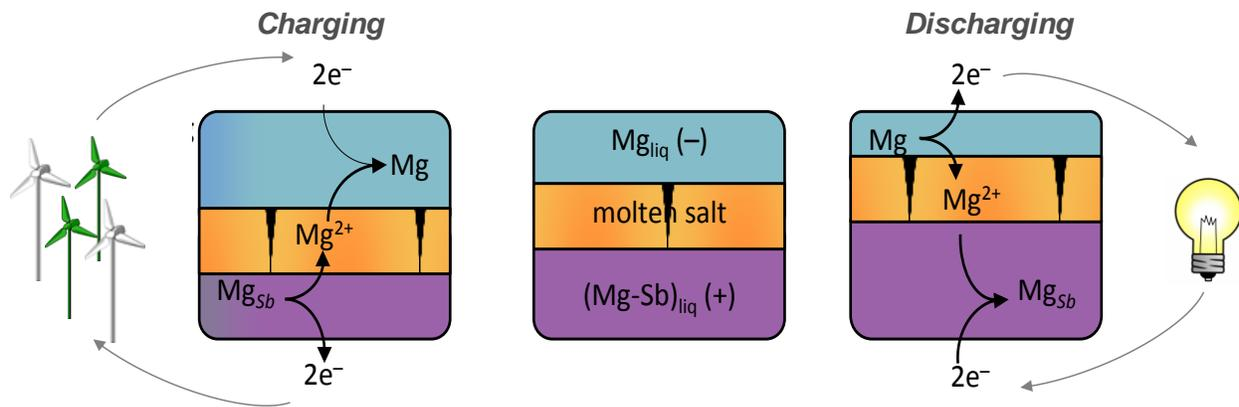
**Fundamentals of the Liquid Metal Battery:** All three main components of the battery are liquid and self-segregate, enabling use of low-cost components that are easy to assemble and will last for a long time.
