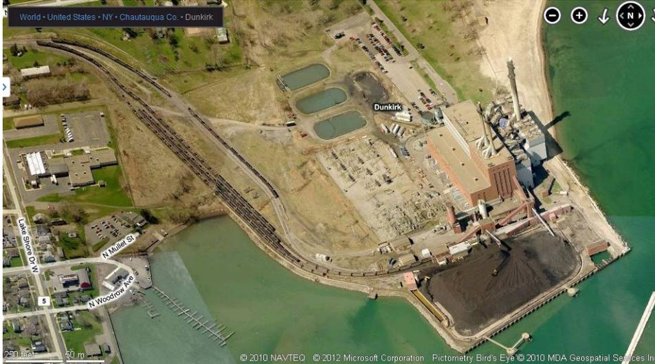
The Dunkirk Station consists of four active generating units with a total nameplate rating of 635 MW net. Units 1 and 2 are identical 100 MW units that began commercial operation in 1950. Units 3 and 4 are identical 218 MW units that went into commercial operation in 1959 and 1960, respectively (Table 1). All Dunkirk units use low-sulfur Powder River Basin coal as their fuel source.
