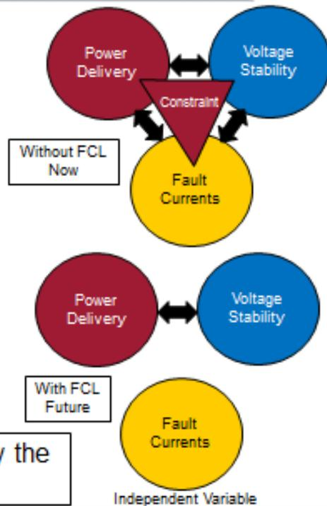
SCFCL's alter the fundamental way the grid can evolve
