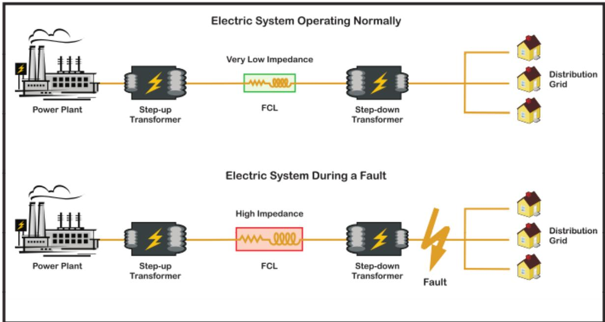
*During a ground fault, an FCL safely mitigates the excess energy that would normally effect utility transmission and distribution equipment, preventing damage.*
